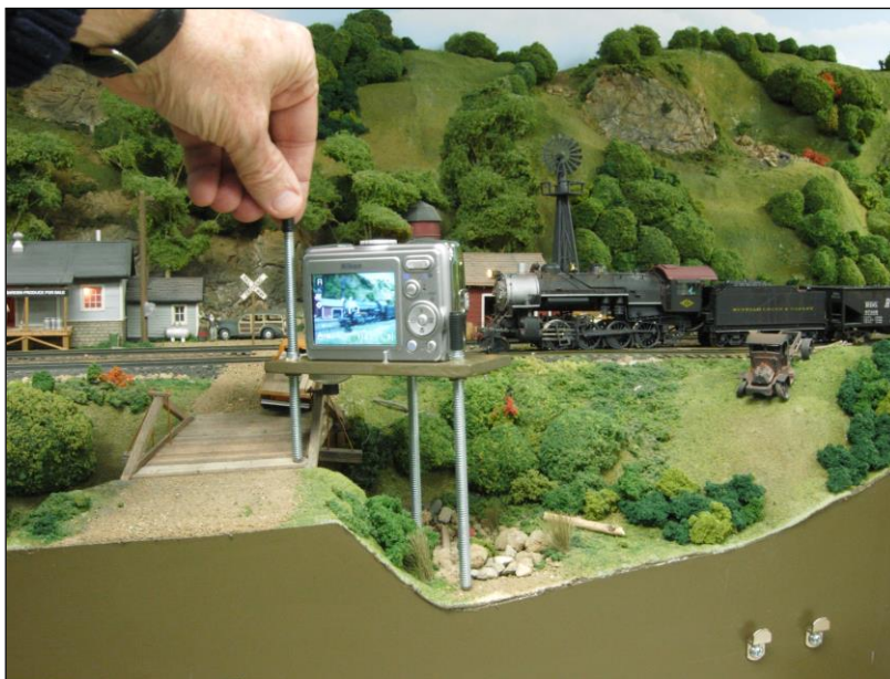
This photo shows the simple tripod I constructed that allows placement of a small point and shoot camera directly on the layout, even where the terrain is irregular. It is made from a small piece of Masonite with internally threaded sleeves installed in the two back corners and the center of the front. The legs are long, threaded carriage bolts that fit in the sleeves. The camera is attached to the unit with a threaded thumb screw. By adjusting the heights of the legs independently, both leveling and precise aiming of the camera is possible.
